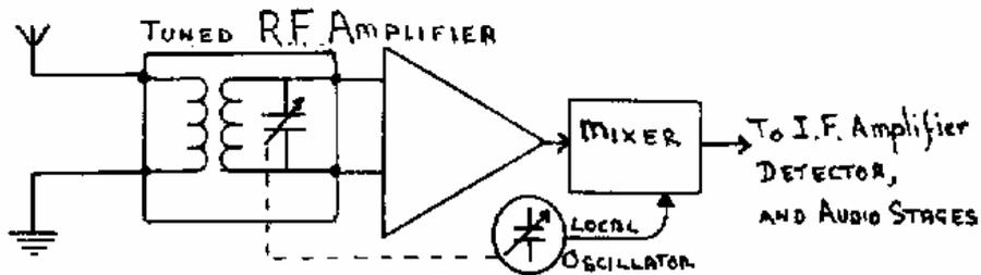
In a superhet there are no feedback problems as a result of using a ganged capacitor as the sections are now operating at different frequencies.
