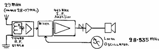
**The Tuned Circuit in the RF Amplifier.**
