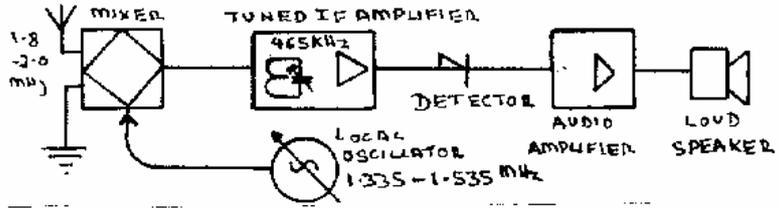
The aerial circuit is connected to one i/p (called local oscillator) is connected to receiver is actually tuned by this oscillator. Superhets for this band would often use an IF amplifier at 465 kHz.
