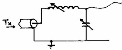
This circuit shows a simple AMU that is being used to match "an end fed wire" to a feeder cable. This AMU can be adjusted to enable the same end fed wire to be used on several Amateur Bands.
