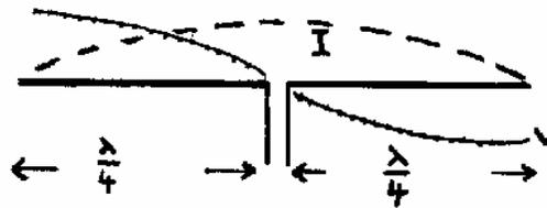
One advantage of this simple aerial is that it has a low impedance at the centre feed point, typically 70Ω or 80Ω. Thus a feeder of that impedance can be used to give a good match and transfer of power.
