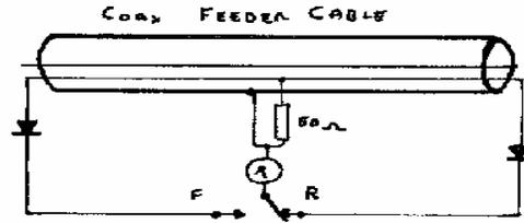
This meter will determine the ratio between the forward and the reverse powers within the feeder cable and can indicate if, for example, the aerial is correctly matched to the feeder.
