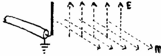
A vertical aerial will create an electromagnetic wave that is said to be vertically polarised. The electric field will be vertical and the magnetic field will be horizontal.
