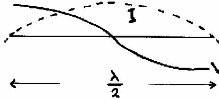
If this *half wavelength wire* is cut in the middle and connected to a radio, it is called a "half wave dipole".
