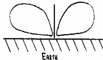
This is the *polar diagram* of a  $\lambda/4$  vertical aerial, as viewed from the sky.. It shows that the signal is radiated equally in all directions, in the horizontal plane – but *vertically polarised*.....
