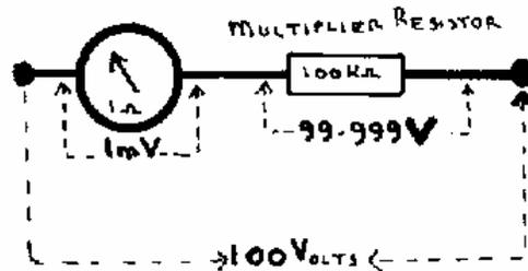
The sensitivity of a meter is quoted in Ohms per Volt. The higher the better but typical good meter would have a sensitivity of 20 kOhm per Volt.
