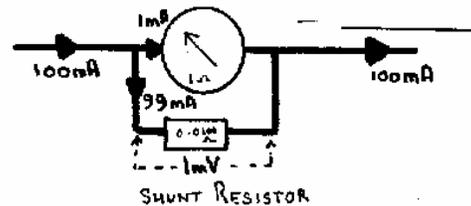
Example. A meter having a FSD of 1mA has a resistance of 1 Ohm. What value of shunt is required to enable currents of up to 100 mA to be measured?
