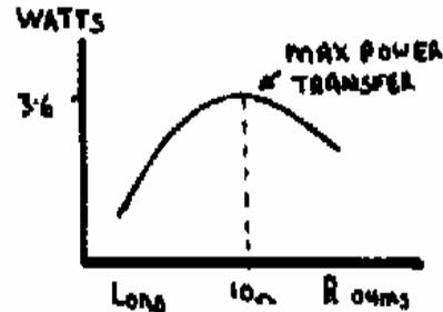
When these results are plotted on a graph it can be seen that most power is dissipated in the load resistor when it is set to 10 Ohms. Note that the internal resistance of the battery was also 10 Ohms....
